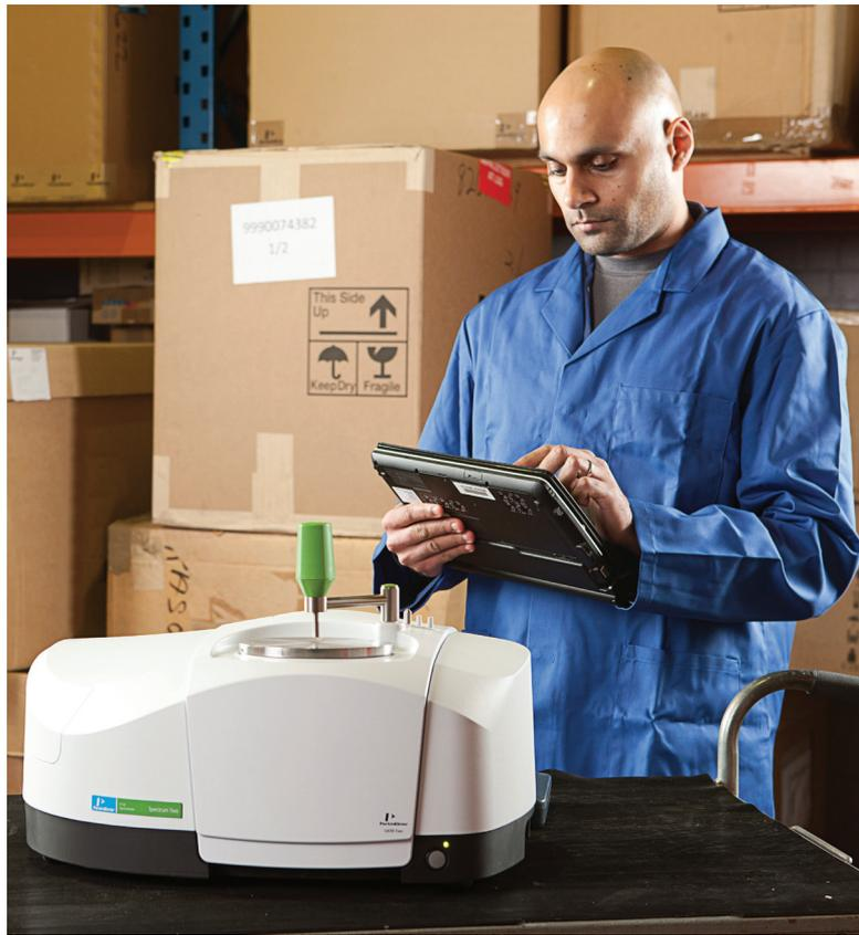
Spectrum Two incorporates a number of features to enable your infrared analysis to move out of the laboratory. Multiple power options allow Spectrum Two to be used with or without external mains power. Once powered, a fast warm-up facilitates rapid measurement while optional wireless connectivity allows portable PC control. Compact and robust, Spectrum Two can easily be transferred from one location to another and the user-install capability allows instruments to be set-up by anyone, anywhere.
