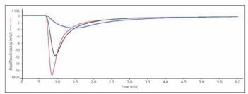
Figure 10. Effect of light intensity with iris opening at 5% (blue), 15% (black) and 25% (pink) at 30 °C on dental resin.
