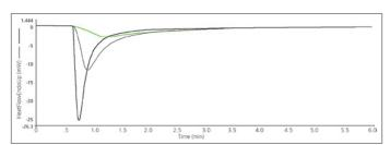
Figure 11. Effect of isothermal temperature at 10  $^{\circ}$  C (green), 30  $^{\circ}$  C (blue), 50  $^{\circ}$  C (black) on dental resin curing with 15% iris opening.
