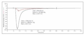
Figure 7. UV curing data at 30 °C with 15% iris, dental resin (red) vs. optical adhesive (black) showing different peak time and energy.
