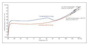
Figure 9. 1st and 2nd heating curves after UV curing, showing residue curing and Tg after that.
