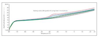
Figure 8. Heating curve after partial UV curing for 0, 0.1, 0.2, 0.3, 0.5, 1, 2 and 4 min, showing the diminishing Tg of uncured material after UV curing.
